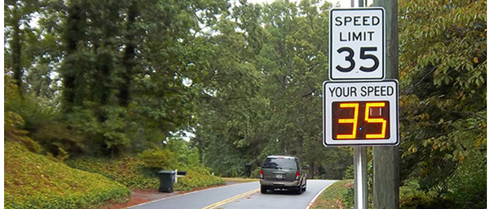
Radar speed signage can be used to promote compliance with the speed limit as drivers can more easily see their driving speed in relation to the speed limit.
